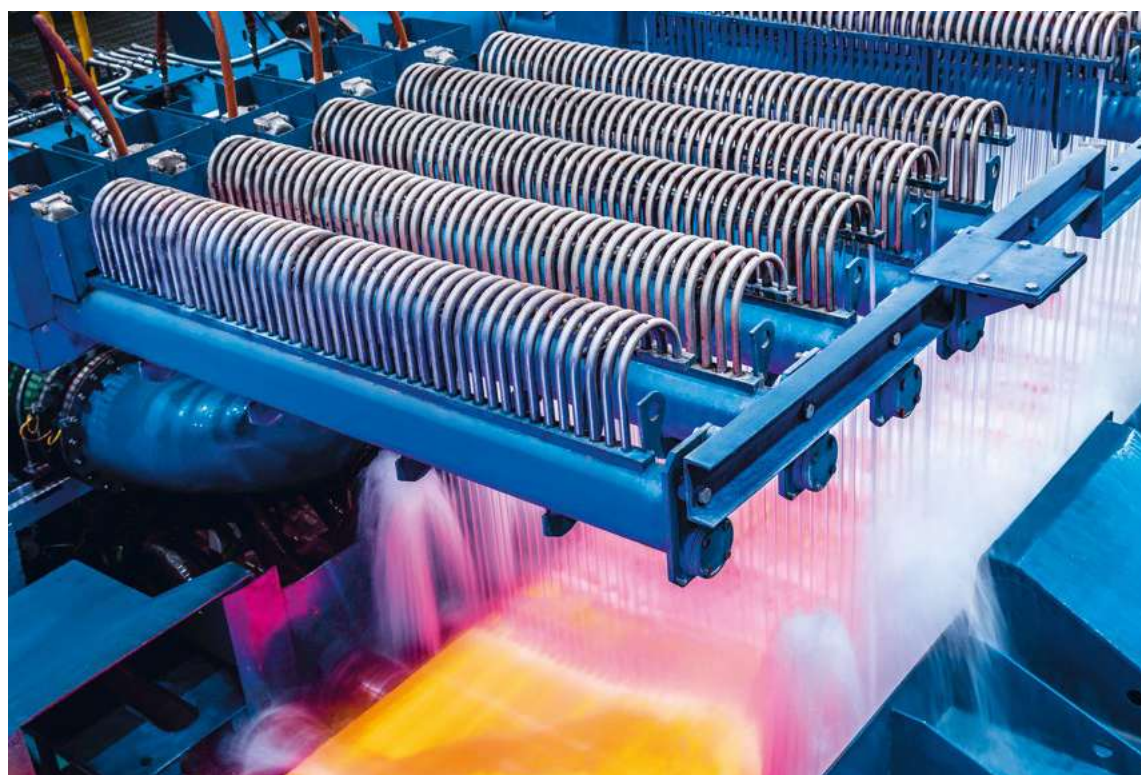
The modernization of the mechanical and automation equipment in the laminar cooling system enables Ningbo to produce new steel grades.
