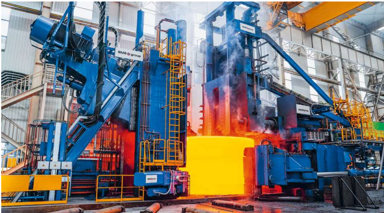
Ring rolling of a shell
