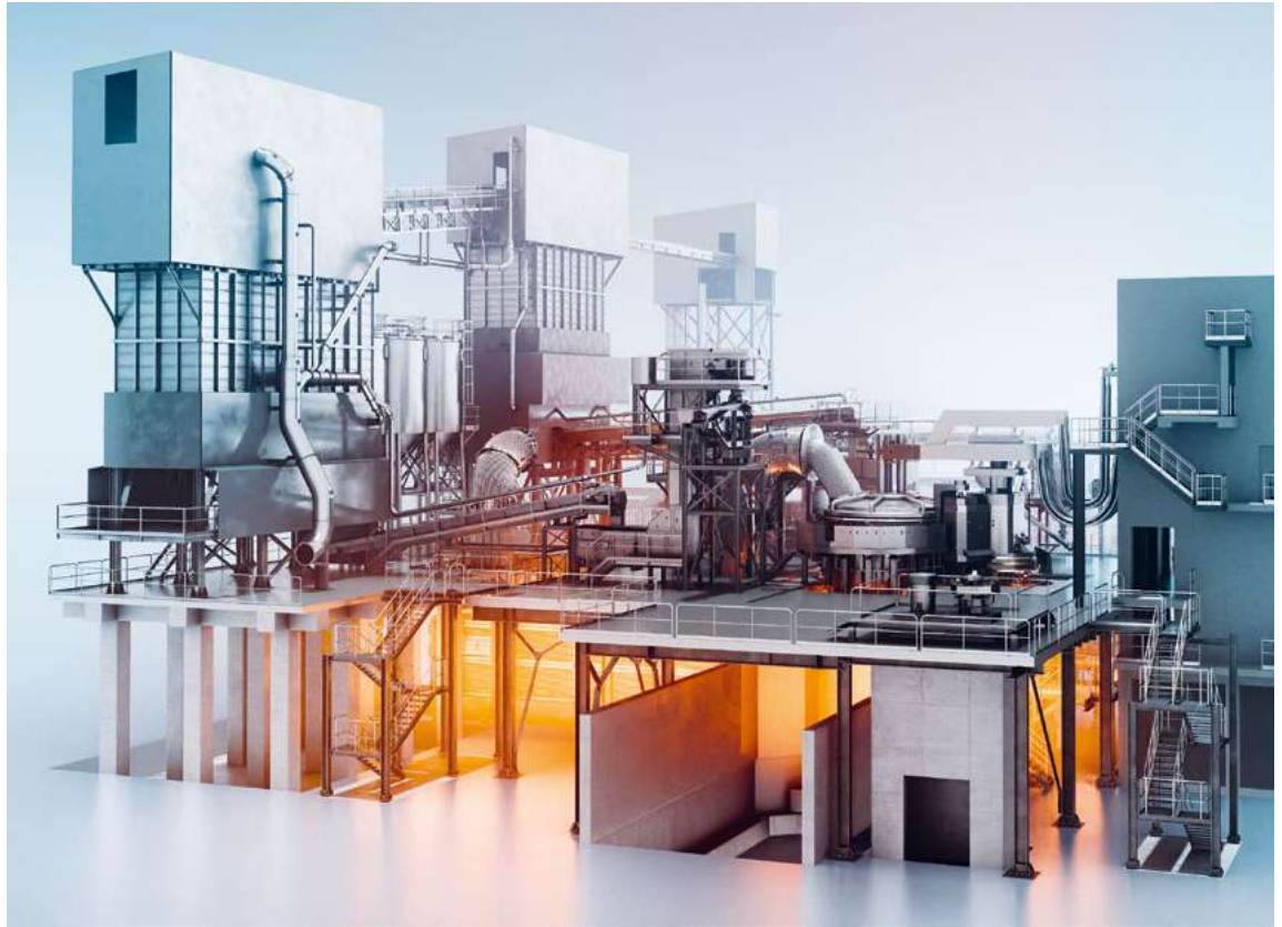
The AllCharge furnace with continuous scrap charging
