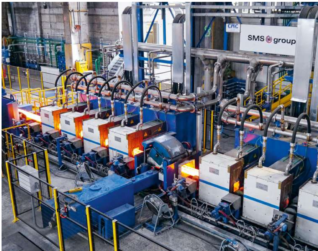
Induction heaters are essential elements in CMT and CSP plants to connect casting and rolling.
