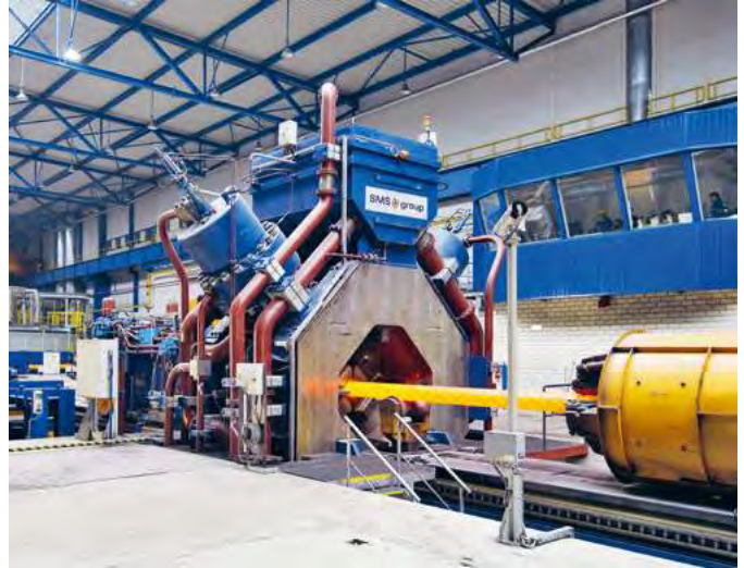
Hydraulic radial forging machine in operation
