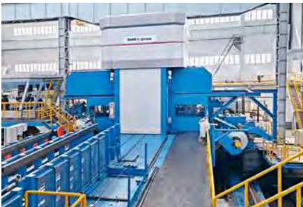
NCA operates a 6-high CVC plus aluminum CRM.
